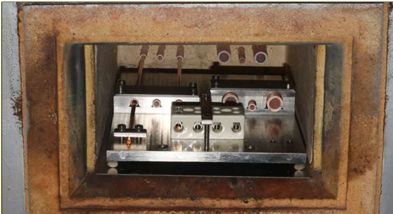
Test oven for the resistivity of ceramics as a function of temperature (Ultimheat Laboratory)
