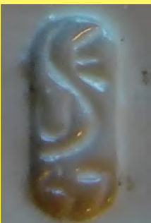
1932 ca USE marking on Maure porcelain terminal blocks
